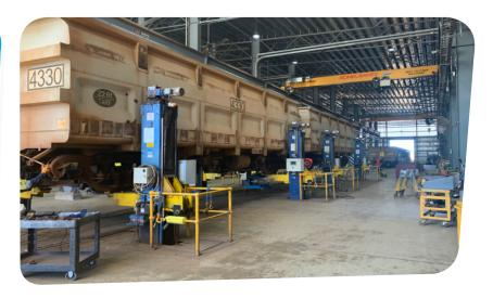
Coastal Electrics provided the installation service & commissioning support for the control systems upgrade on jack systems OP1200 & OP1400. This included the installation of LV cabling, ELV cabling, communications cabling, migration of existing Eurogamma system to Siemens PLC and PLC panel fabrication.
